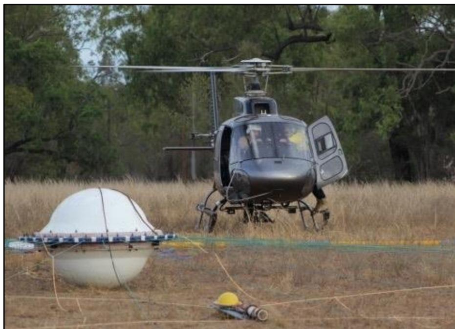
Figure 2 – Helitem<sup>2</sup> system with large diameter ‘Fat Boy’ receiver shown in foreground
