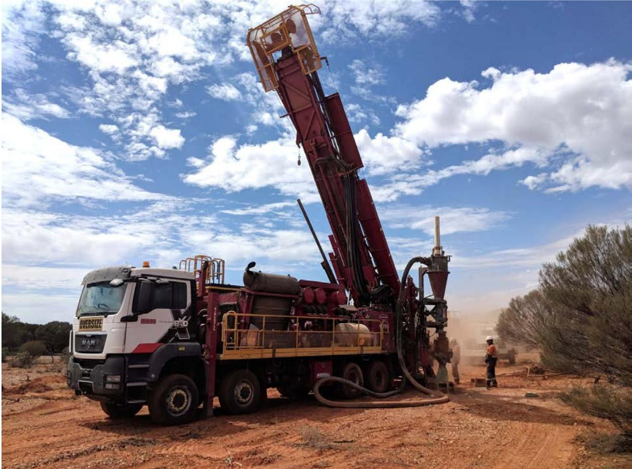
*Figure 1: Reverse Circulation (RC) drill rig at the Centauri prospect, where drilling commenced in March 2019.*
